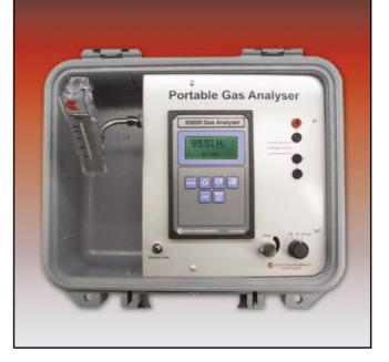
A large, alphanumeric LCD shows measured values and also displays messages and prompts for the menudriven configuration and calibration routines. These procedures are simple and straightforward.
