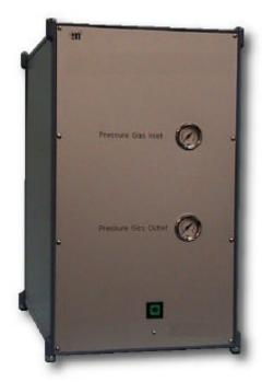
Max. air inlet temperature + 30 °C. Air should be prefiltered and oil free. To guarantee a longlasting maintenance-free use please use air with the following standards: ISO 8573.1, class 1.2.1. Oilcontent < 0,01 mg/m³, water content < - 40 °C dew point, particles < 0,1  $\mu$ m. In case of dirty compressed air with maybe high rate of oil and water special coalscing-filters can be delivered.
